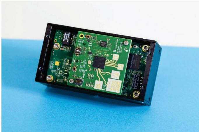
The innovative sensor solution of "RoKoRa" consists of 16 radar modules, each made of a 77 GHz front end from Fraunhofer IAF.
